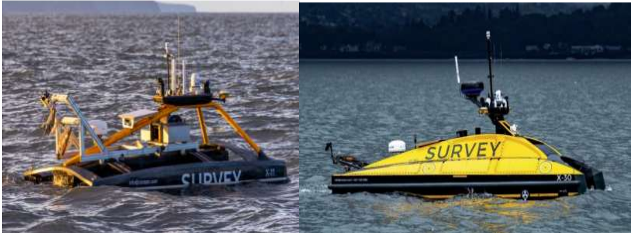
Figure 3: USV with towed sensors
